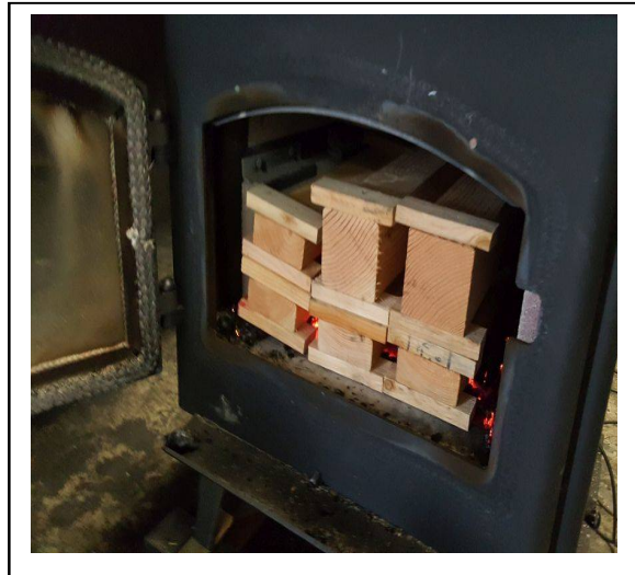
Run 8 – Newly Loaded Stove
